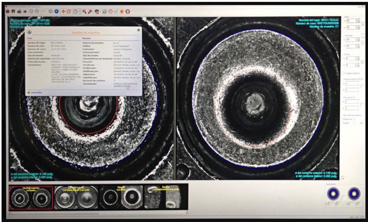
The IBIS computer rendition of a bullet's fingerprint at the Attorney General's Ballistic Unit office. (Photo credit: Steven Dudley)
